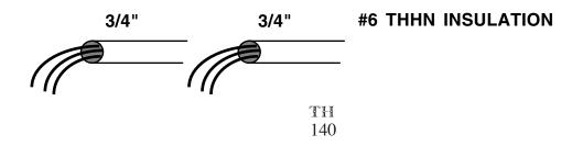
II. Single conduit run to the machine. Both branch circuits to the two motors on the machine could be carried in a single conduit. The *variable* for more than three current carrying conductors would affect the wire size in this case.
