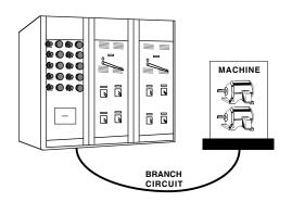
Example: A machine has two 15 hp, 230v, 3ø squirrel-cage induction motors. Each motor is fed by a *separate* branch circuit originating at a combination motor controller in a motor control center. Rigid steel conduit is to be used, assume ambient not over 86°F, and voltage drop is limited to 3%. 60°C equipment.
