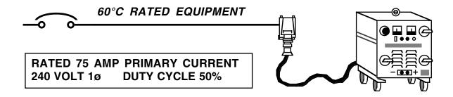
Wire size: Table 630.11(A) lists a multiplier of .71 for a 50% duty cycle. The rated primary current 75a x .71 = 53.25 required ampacity. Table 310.16 shows a #6 THHN has an ampacity of 75 amps, but connected to  $60^{\circ}$ C equipment a #6 THHN can be loaded to 55 amps. The required ampacity is 53.25 amps so a #6 THHN would meet the Code requirements.
