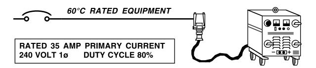
Wire size: Table 630.11(A) lists a multiplier of .91 for a 80% duty cycle. The rated primary current  $35a \times .91 = 31.85$  required ampacity. Table 310.16 shows a #8 THHN has an ampacity of 55 amps, but connected to 60°C equipment a #8 THHN can be loaded to 40 amps. The required ampacity is 31.85 amps so a #8 THHN would meet the Code requirements.
