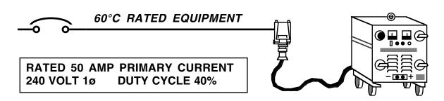
Wire size: Table 630.31(A2) lists a multiplier of .63 for a 40% duty cycle. The rated primary current 50a x .63 = 31.5 required ampacity. Table 310.16 shows a #8 THHN has an ampacity of 55 amps, but connected to  $60^{\circ}$ C equipment a #8 THHN can be loaded to 40 amps. The required ampacity is 31.5 amps so a #8 THHN would meet the Code requirements.
